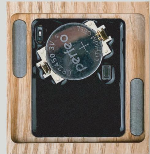
The **BeeSwitch** is powered by a battery (CR2450), so no need for an electrical box for installation. All you have to do is to install a mounting plate with two screws (supplied) to the surface where the switch should be.
